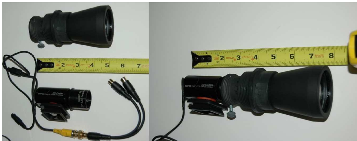
Figure 4 – Mighty Mini video camera and objective lens system. The measuring tape shown is in units of inches.
