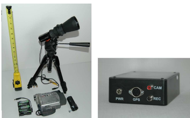
Figure 5 – Complete Mighty Mini system with imager, recorder, power and GPS.
